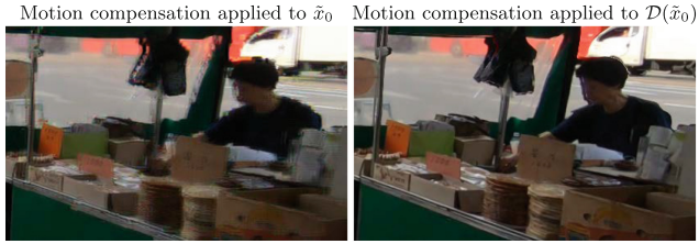
Fig. 4. Comparison between applying motion compensation to \tilde{x}_0 in the latent space and to \mathcal{D}(\tilde{x}_0) in the pixel domain. \mathcal{D} represents the VAE decoder. In the first scenario, visible artifacts are introduced.
