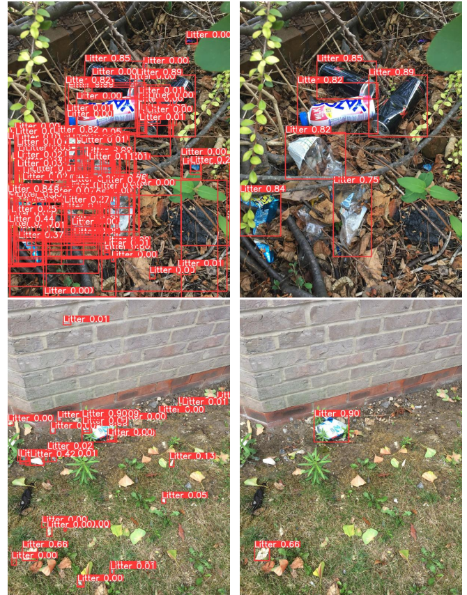
Fig. 1. Qualitative evaluation of the effect of the modification of the confidence threshold from the default value conf = 0.001 (left) to a higher value conf = 0.5 (right).
